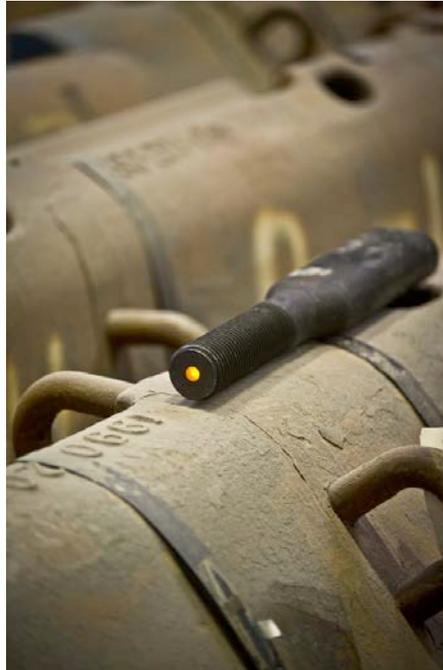
Figure 5 – The iBolt showing the elongated head and indicator light
