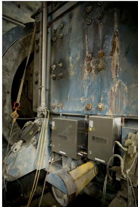
Figure 2 – MCU Control boxes mounted on the side of the feed chute
