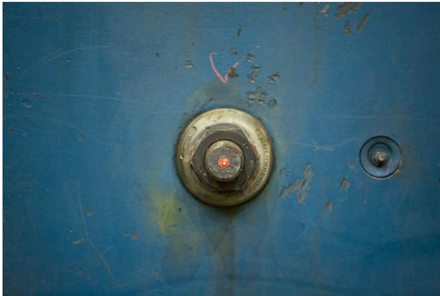
Figure 4 – An activated iBolt installed on the shell of a SAG mill
