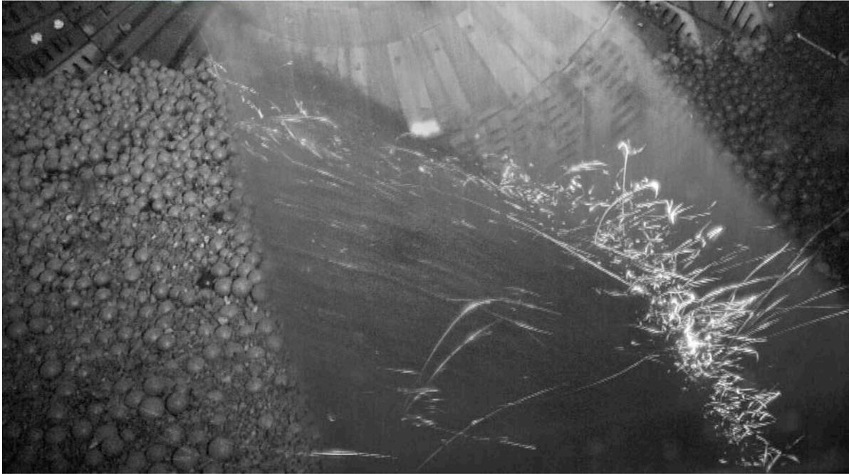
Figure 7 – Composite image showing the toe of the charge in the 38’ SAG mill at Canadian Malartic at approximately 7.5 rpm overlaid with the stationary charge position
