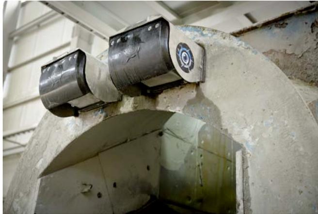
Figure 1 – MCU Camera and lighting housings mounted on the feed chute flange
